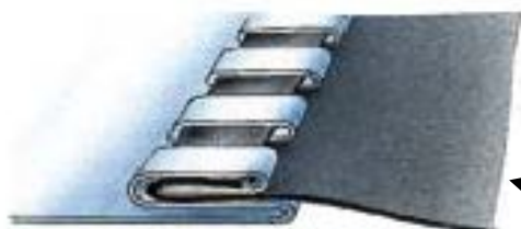
Seam Type LOC-4 Steel 28 ga. (0.4mm) Many dimensions
